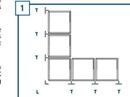
**UK** Cut the tabs of a cross into an "L" shape (for the starting angle) or "T" shape (for the first row of blocks) (photo 4 and figure 1).
